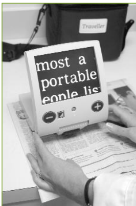
The Traveller magnifier can give 16X magnification
