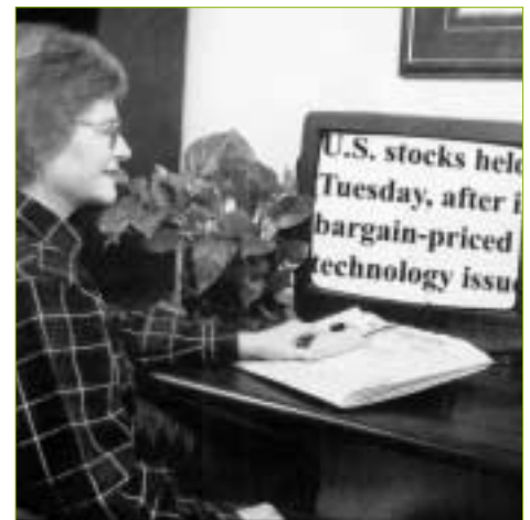
Low vision patient uses a portable digital magnifier which connects to a television or computer to enlarge the printed page.
